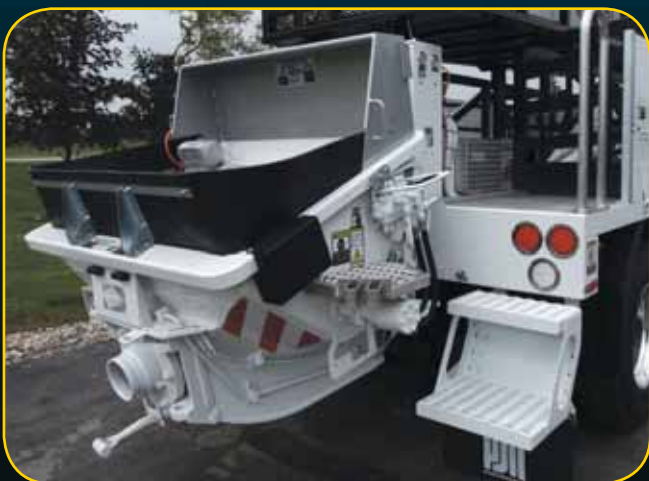
Large capacity hopper and breakaway rear steps
