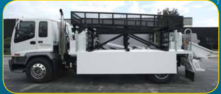
Deck-mounted pipe racks shown with optional overhead pipe rack
