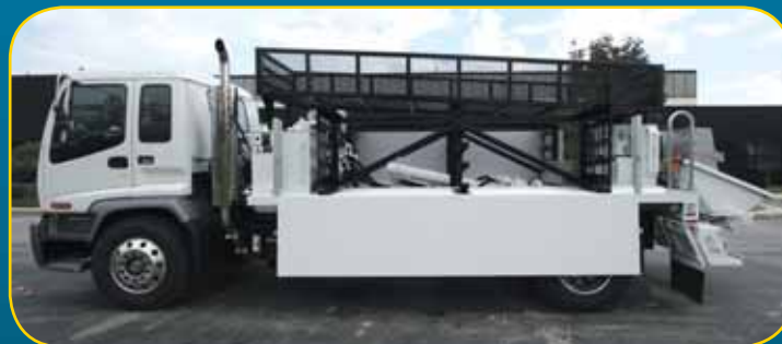
Deck-mounted pipe racks shown with optional overhead pipe rack
